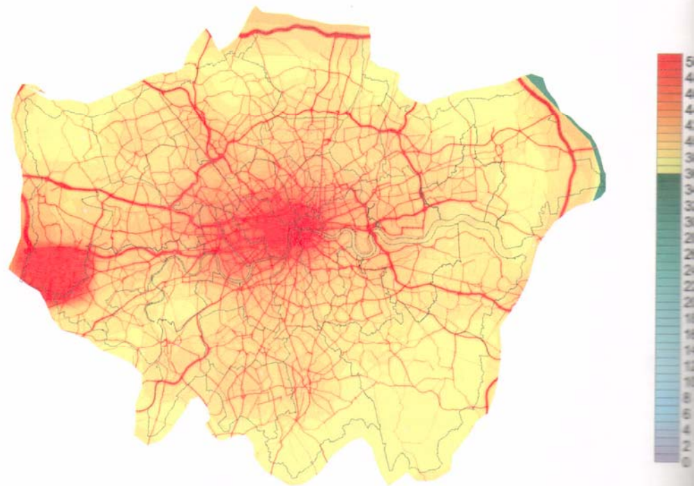
figure 16 Modelled 1999 daily average PM_{10} concentrations, in number of days exceeding the national objective level
